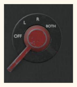
**Ignition Switch:** The "Magnetos" (self-contained generators) power the spark plugs. Depending on switch position either none, left, right or both banks of plugs are powered.
