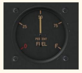
**Fuel gauge:** Shows the remaining capacity of a fuel tank in percent. There are 3 fuel gauges on the Tomahawk. One on the main panel, and the floor mounted ones for both wing tanks.
