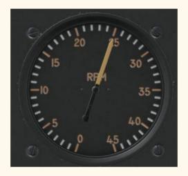
**Propeller Speed:** This shows the revolutions of the propeller in hundreds per minute.
