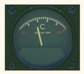
**<u>Radiator Temperature:</u>** Shows the engine coolant temperature in degrees Celsius (°C).
