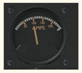
**Loadmeter:** Shows the load put on the generator by the electrical system in Ampere.
