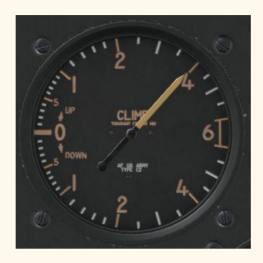
**<u>Vertical Speed Indicator:</u>** Indicates your vertical speed in thousands of feet per minute.
