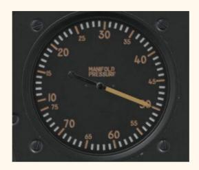
**Engine Manifold Pressure:** This indicates the manifold pressure (MAP in short) in inch Hg.
