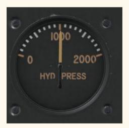
**Hydraulic Pressure:** The pressure of the hydraulic system used for flaps and gear in PSI.
