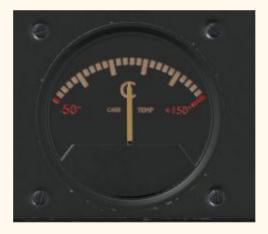
**Carburetor Temperature:** Shows the temperature inside the carburetor body in °C.
